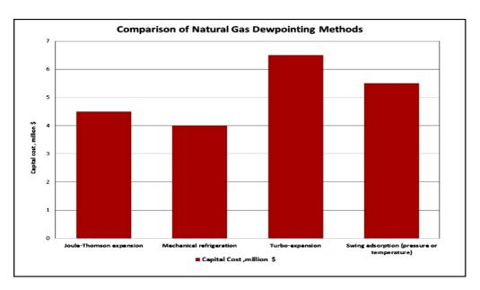
Figure 8: Capital Cost for different natural gas hydrocarbon dew pointing control methods
