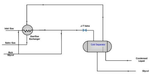
Figure 1: PFD for a typical Joule-Thomson Expansion unit [7]
