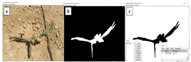
Figure 2. Digital image processing to estimate canopy cover for O.ficus-indica plant. a: cropped image to center and delimitation of green canopy cover, b: converting to binary image with 8 bits, c: determination of area of interest. Estimated CC=~5.23%
