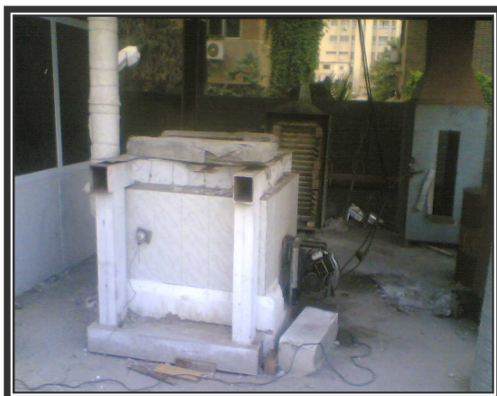
Fig (1) Test setup of fire furnace
