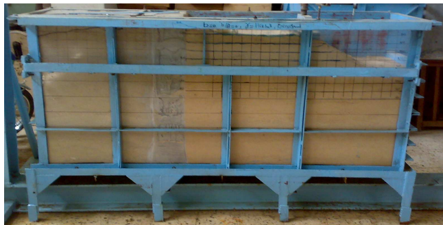
Photo. (1): Sand container (Tank model)
