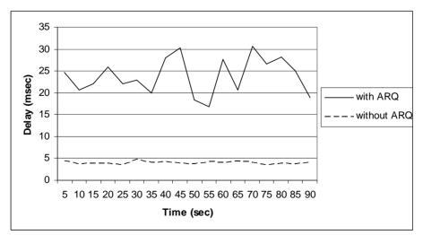
Figure 3- Video delay with and without ARQ
