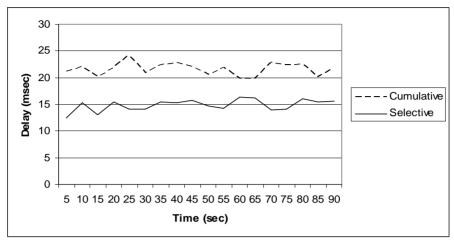
Figure 8 – Effect of ARQ ACK types on delay.
