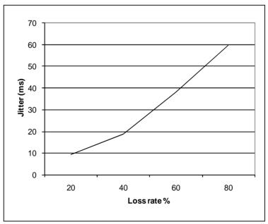
Figure 5- Relation between loss rate and jitter.
