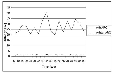
Figure 4- Video jitter with and without ARQ
