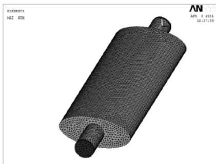
Fig. 2. Typical FE model of an elliptical expansion chamber
