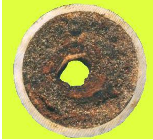
Figure 0: Deposition of wax in oil pipelines
