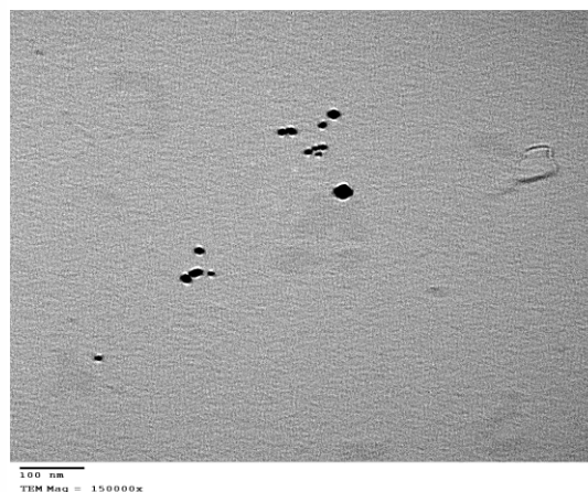
Fig.2: TEM image of the prepared Ag NPs particles in the polymer matrix
