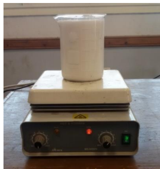
Fig. 2 AL_2O_3 magnetic stirring
