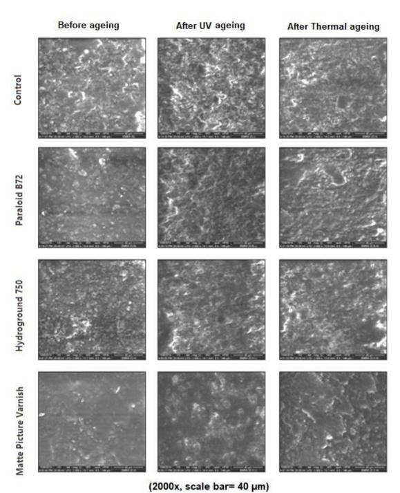
Fig. 7. FE-SEM micrographs (2000x, scale bar =  $40\mu m$ ) of the treated green painted samples before and after UV/thermal ageing
