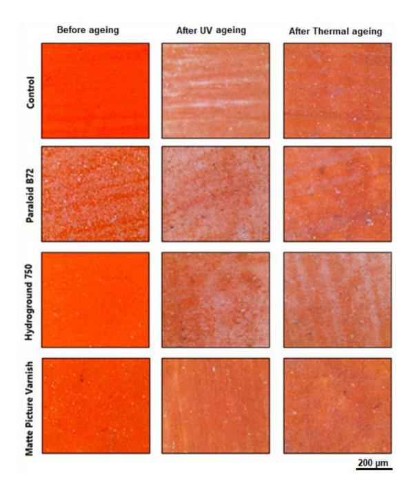
Fig. 2. Microscopic images (at magnification 100 X, scale bar=200µm) of the appearance of red painted models before and after UV/thermal ageing.
