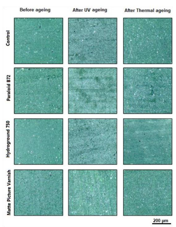
Fig. 3. Microscopic images (at magnification 100 X, scale bar=200 $\mu$ m) of the appearance of green painted models before and after UV/thermal ageing.
