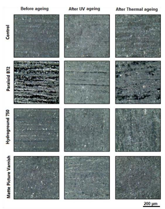
Fig. 4. Microscopic images show (at magnification 100 X, scale bar=200µm) the appearance of black painted models before and after UV/thermal ageing.
