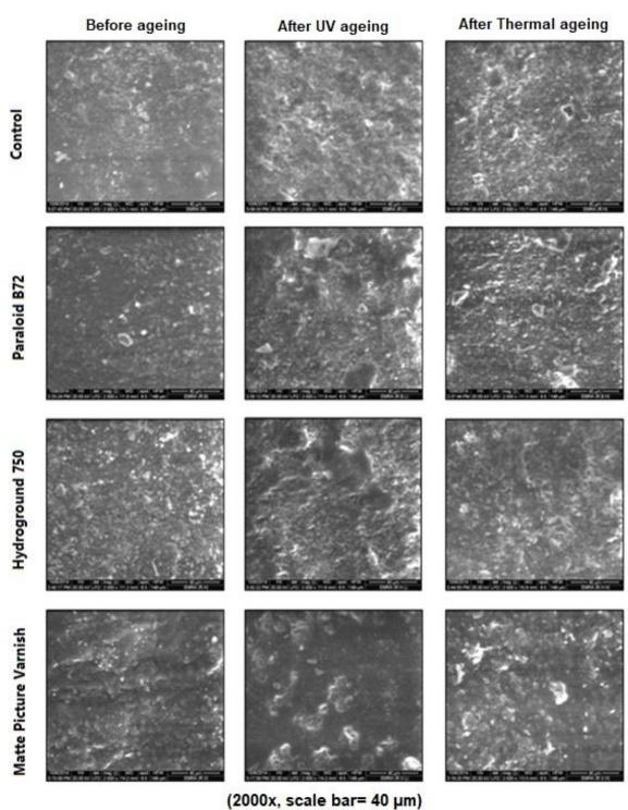
Fig. 6. FE-SEM micrographs (2000x, scale bar =  $40\mu$ m) of the treated red painted samples before and after UV/thermal ageing.
