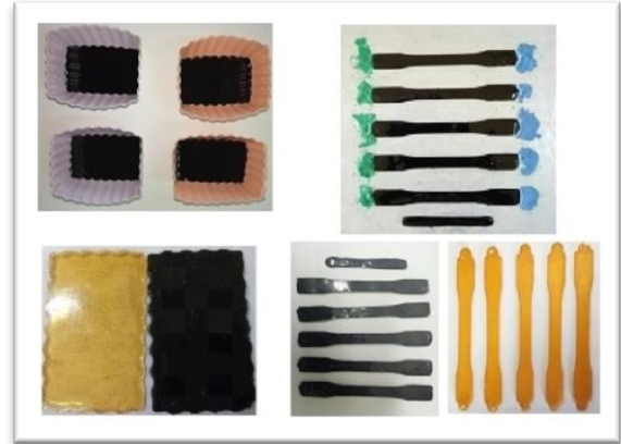
Figure (1): The aluminum mold and silicone pans used for molding the samples
