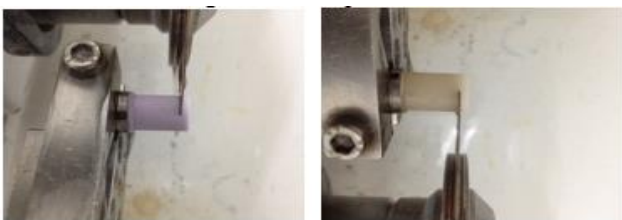
Fig.2 Disc fabrication using IsoMet 4000 micro saw
