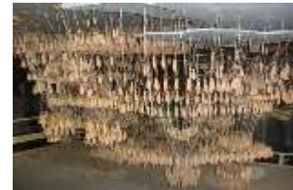
Fig-2 Funicular chain string model of Colonia Güell church project by Gaudi.
