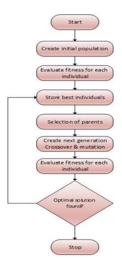
Figure (9) Flow chart for the genetic algorithms technique
