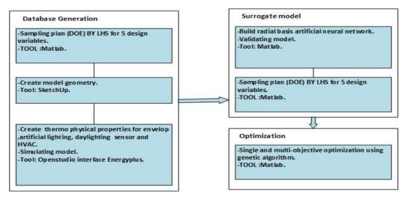
Figure (4): A flowchart of the surrogate-based optimization approach
