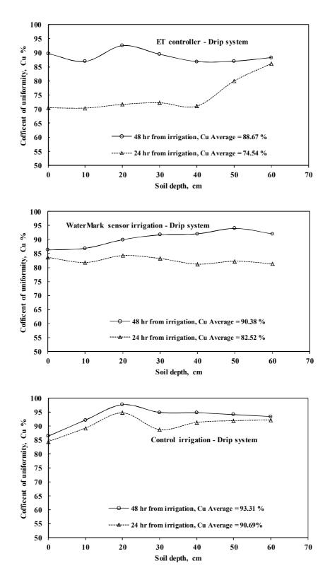
Fig. 2. Values of Cus as a function of soil depth after 24 and 48 hours of irrigation, for the three irrigation-scheduling methods
