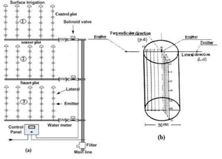
Fig. 1. Field experimental layout (a) and diagram showing sampling for soil moisture contents parallel and perpendicular to the direction of the irrigation line (b).
