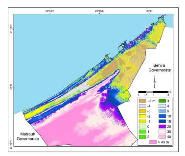
Figure (4). DEM for Alexandria City using ASTER data and IDW technique
