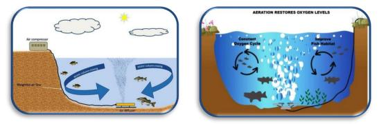
Figure (7): Artificial Aeration System (www.Watergardengems.com)
