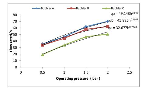
Fig. 2. Calibration of bubbler
