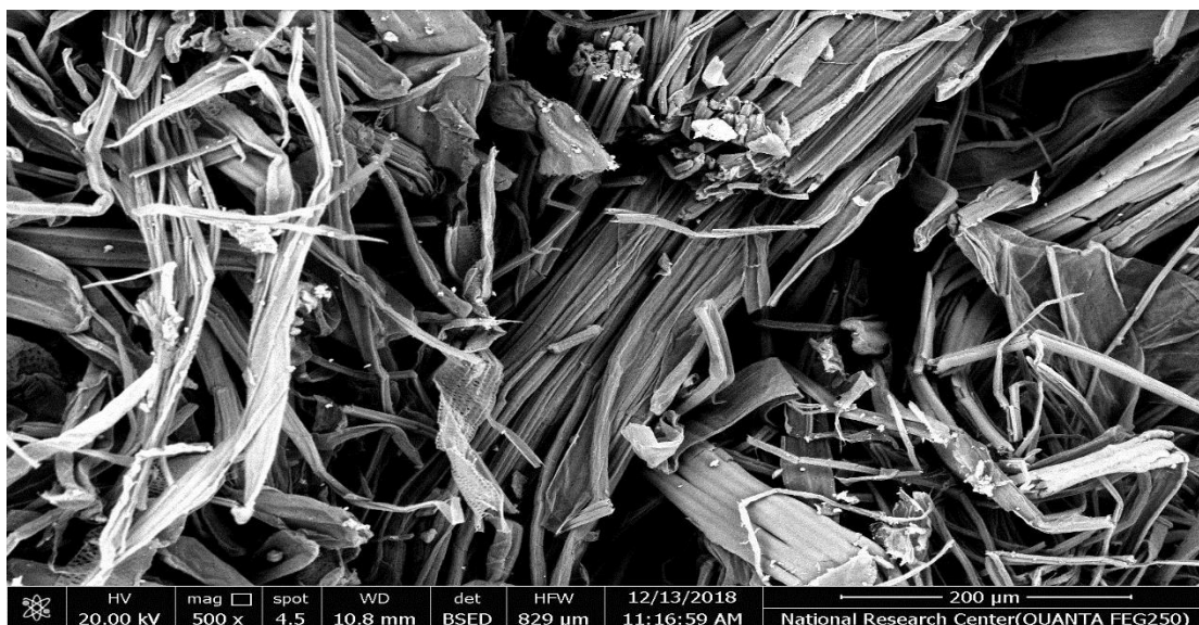
Fig.1. SEM Scan of corn stalk fiber, magnification 500 x
