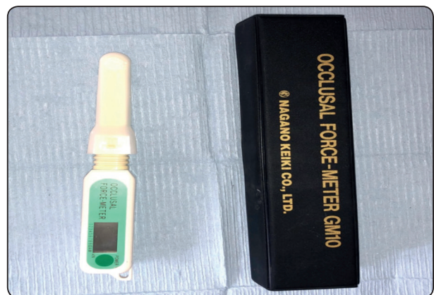
Fig. (4): A photograph showing the occlusal force-meter GM10 associated with a disposable plastic cap and storage case.
