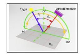
Fig.3. The Measuring geometry, Illumination angle ( $\theta$ i), Viewing angle ( $\theta$ v) and Rotating angle ( $\theta$ w).
