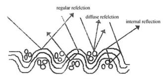
Fig .1 Schematic diagram light reflection from surface of textile.
