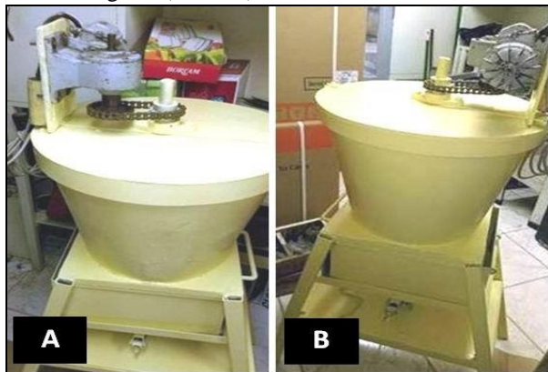
Figure 2. (A and B) The prototype parts with power transmission unit.
