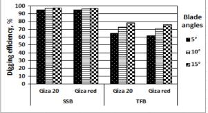
Fig. 6. Effect of blade type and blade angle on digging efficiency during digging the two onion cultivars Power requirement and consumed energy:-
