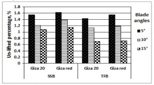
Fig. 4. Effect of blade type and blade angle on the unlifted bulbs percentage for the two onion cultivars
