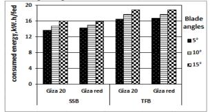
Fig. 8. Effect of blade type and blade angle on energy consumption for the two onion cultivars
