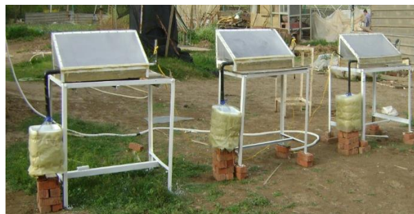
Fig. 2. Three identical passive single-slope solar stills.
