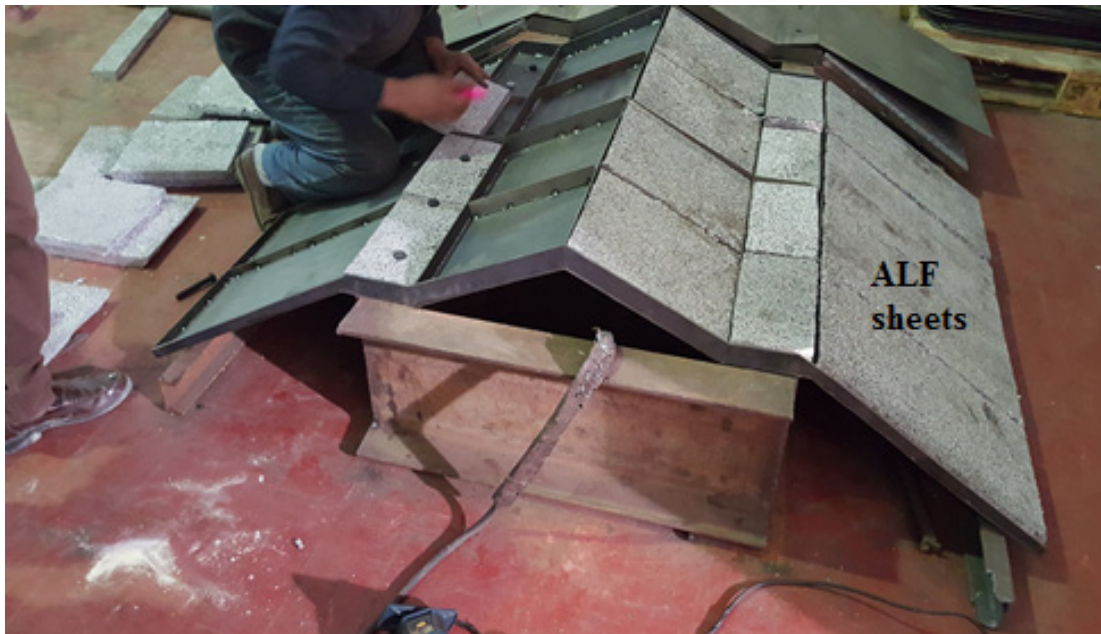
Fig. 3: The use of ALF as a filling material for the V-shape composite structure (after Mazek et al. [1] )
