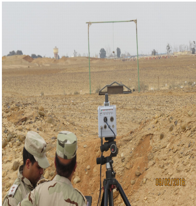
Fig. 5: High speed camera used in the field blast test (after Mazek et al. [1] )
