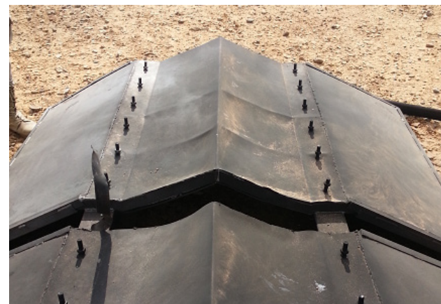
Fig. 7: Test specimen strengthened by the steel cross ribs and ALF after explosion (after Mazek et al. [1] ).
