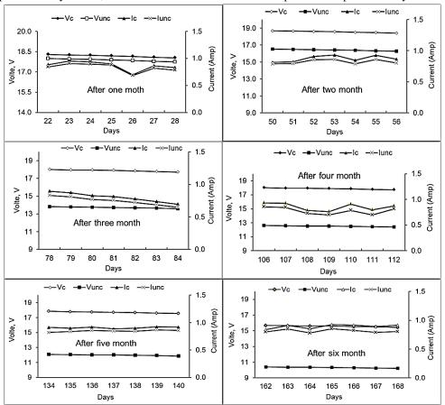
Fig. 5. Variation of current and voltage for the cleaned and un-cleaned surfaces after two to six months of dust deposition
