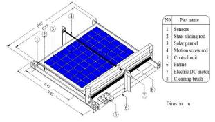
Fig. 1. Solar panel cleaning system
