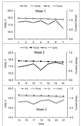
Fig. 4. Variation of current and voltage for the cleaned and un-cleaned surfaces after one to three weeks dust deposition.
