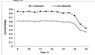
Fig. 7. Variation of current for the cleaned and un-cleaned panels at the end of dust deposition period (168 days).
