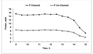
Fig. 8. Variation of power for the cleaned and un-cleaned panels at the end of dust deposition period (168 days).
