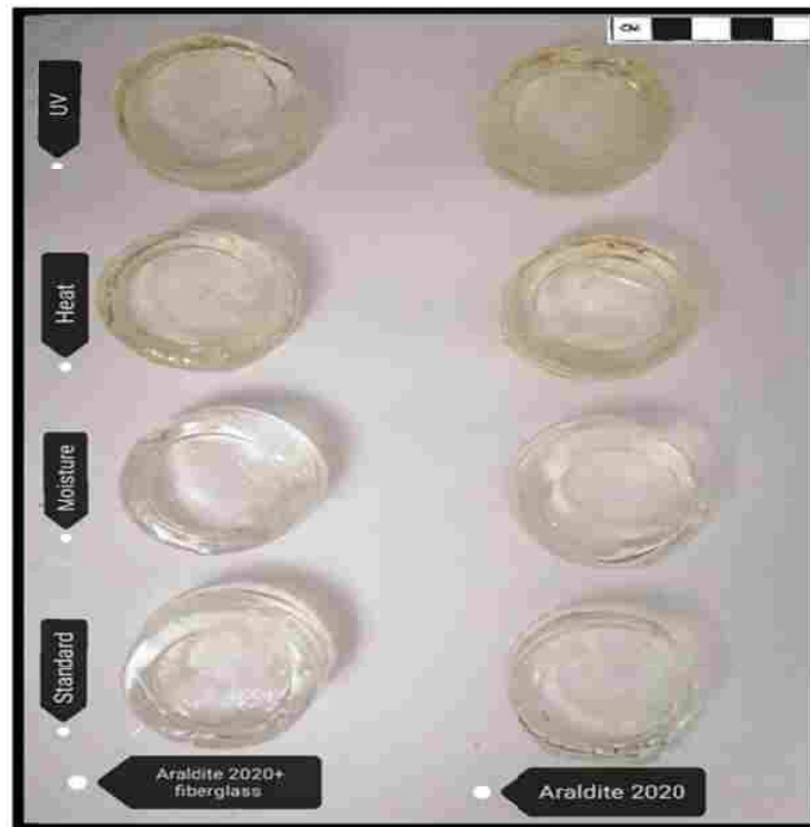
Fig.5, Samples of Araldite 2020 and Araldite 2020 + Fiberglass before and after moisture, thermal and UV ageing.
