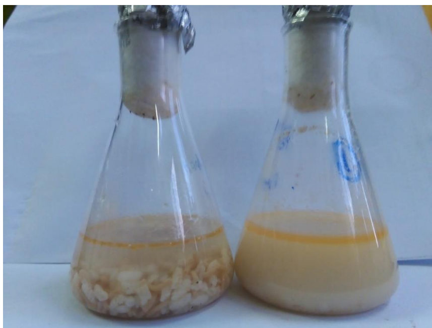
Figure 2: Biodegradation of cooked rice grains by an α-amylase enzyme. The left flask is untreated rice grains and the right flask is the treated rice grains.
