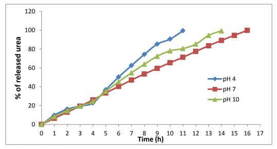
Figure (2): The release rate of urea from CRUF5 in different media.
