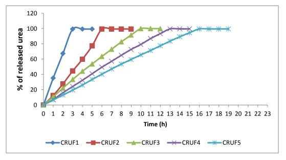
Figure (1): The release rate of urea from different CRUF formulations in distilled water.
