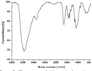
Figure 2: IR spectrum of chitosan in the region  $400-4000 \text{ cm}^{-1}$ .
