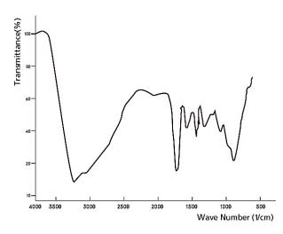
**Figure 4:** I.R spectrum of O-carboxymethyl chitosan in the region 400-4000 cm<sup>-1</sup>.
