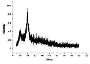
Figure 3: X-ray diffraction of chitosan.
