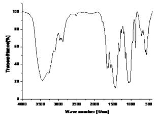
Figure 1: IR spectrum of chitin in the region 400- $4000 \text{ cm}^{-1}$
