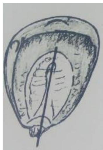
Fig. 2. Grain preparation before testing(cut longitudinally).
