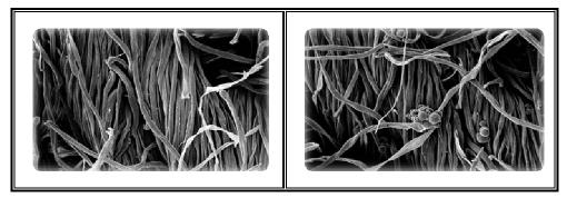
Fig. 4: (A) Control cotton fiber and (B) cotton fiber embedded with gelatin/vitamin D microcapsules.
