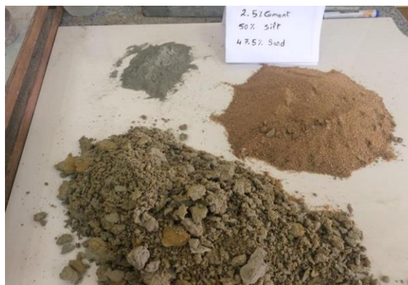
Fig. 2. Sample of CSEB mix ingredients.
