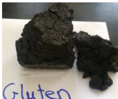
Fig. 8. Failure of Bitumen and Gluten Specimens due to water absorption.
