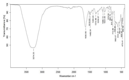
Fig. 3. FT-IR analysis of silver nanoparticles synthesized using A. sakultaensis mycelial free filtrate
