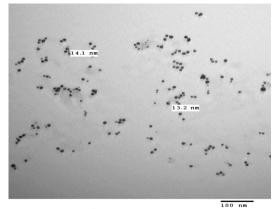
Fig. 2. Transmission electron microscopic image of spherical shaped silver nanoparticles 5-25nm in size [scale bar=100nm]
