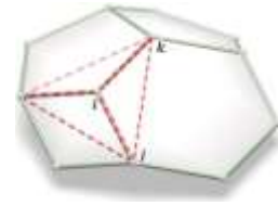
Fig. 4: A mixed polygonal mesh. The vertex star around vertex i consists of all triangles generated by the edges through i .
