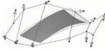
Fig. 3: The control points of a ruled B-spline surface are displaced to optimally approximate a given point cloud.
