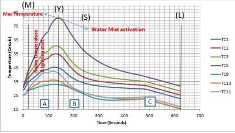
Figure 9 Fire Test with Conventional Nozzle (Viking)
