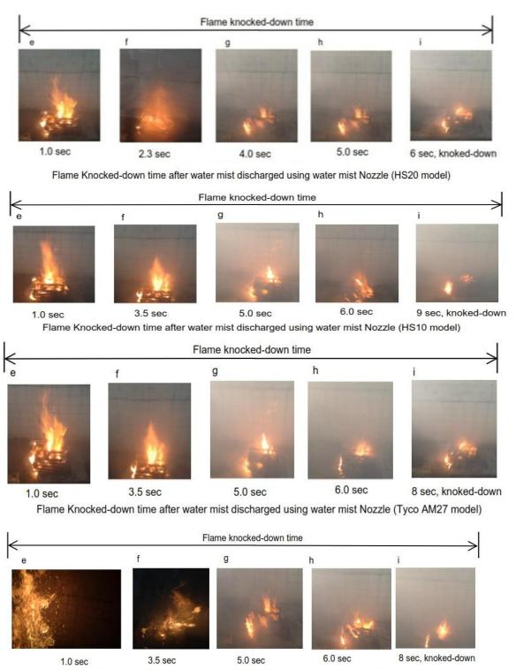
Flame Knocked-down time after conventional system discharged using Conventional sprinkler (Viking model)
