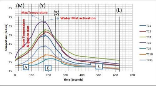
Figure 7. Fire test with LPWM nozzle (HS10 Nozzle)
