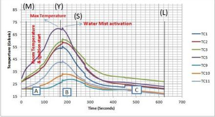
Figure 6 Fire test with LPWM nozzle (HS20 Model)
