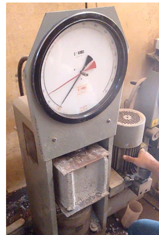
Fig (3): Compressive strength test Source: researcher
