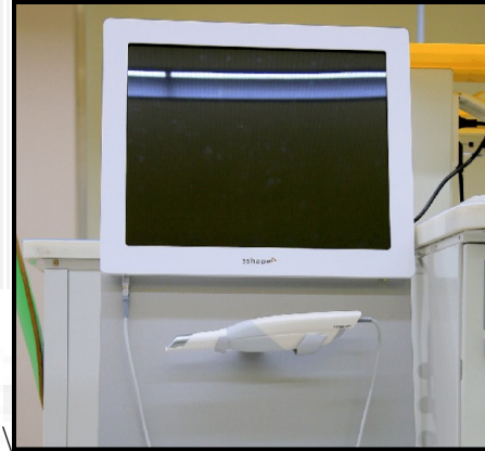
Figure (1): Intraoral scanner 3shape TRIOS basic scanner for obtaining three-dimensional data.
