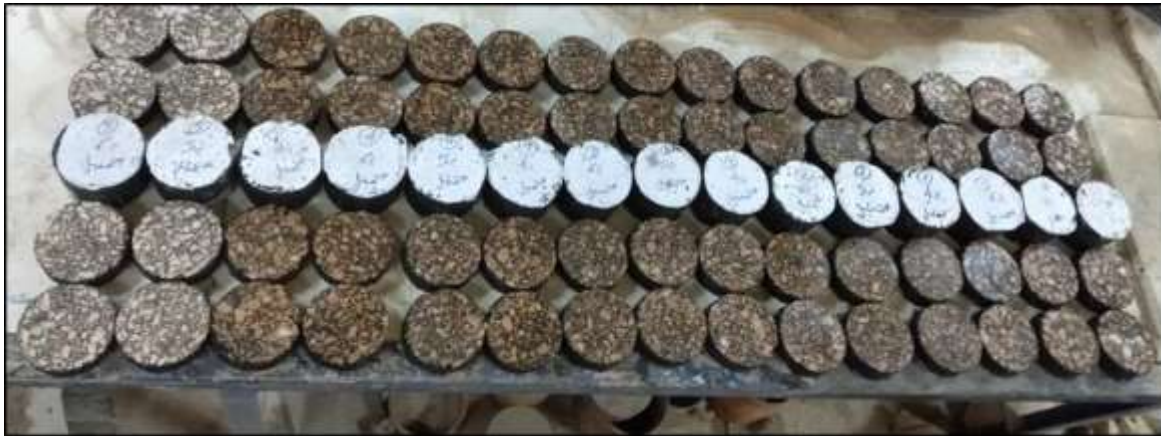
Figure 8: Asphalt samples after cutting.
