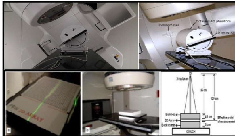
Figure (4): 2D Array for IMRT and VMAT plan verification with Octavius 4D phantom and its setup indifferent measurement techniques
