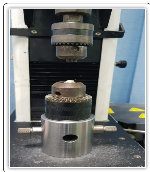
FIG (1) The sample on universal testing machine for tensile bond strength testing
