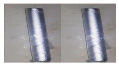
Fig. 1 Aluminum foil mold in cylindrical shape.
