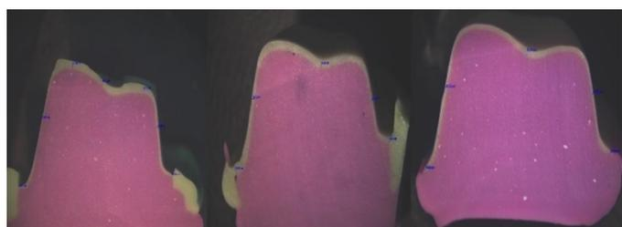
Marginal adaptation difference between CAD/CAM systems. **Figure 4:** Replica measurement for CEREC, CERAMILL & ZIRKONZHAN groups.
