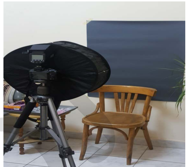
Fig. (1): (The mini studio) Nikon D3400 DSLR camera with 18-55mm VR lens, Godox VING V860IIN Flash for Nikon, collapsible magnetic ring softbox, adjustable tripod stand, and natural gray cardboard background
