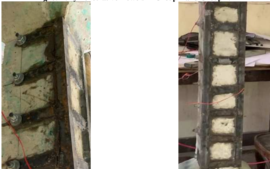
Fig. 7: Welded Connections between Angles and Steel Stirrups.
