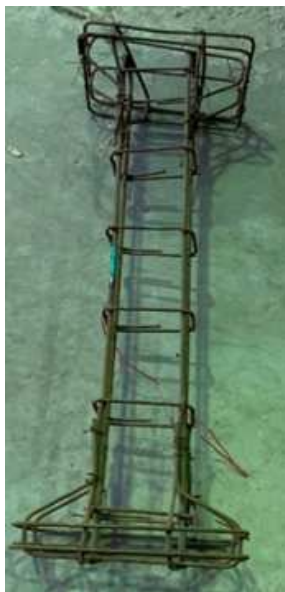
Fig. 3: Reinforcement of Columns in Group (1)
