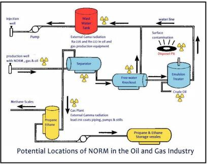
Fig.2 Potential locations of NORM in the oil and gas industry
