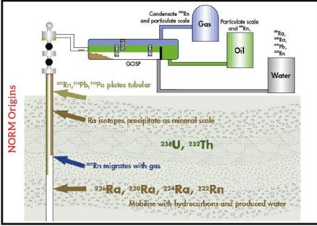
Fig.1: NORM Origins [2] (Adapted from OGP, 2008)
