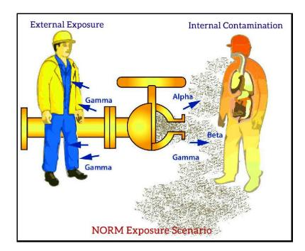
Fig.4: NORM Exposure Scenario [2] (Adapted from OGP, 2008)
