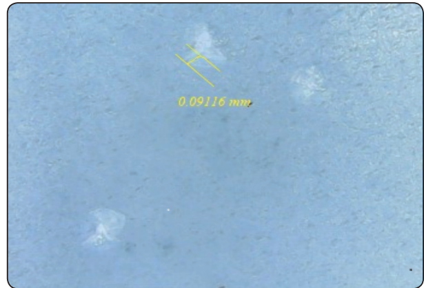
Fig.(1): Microscopic image of indentation crack showing crack extension
