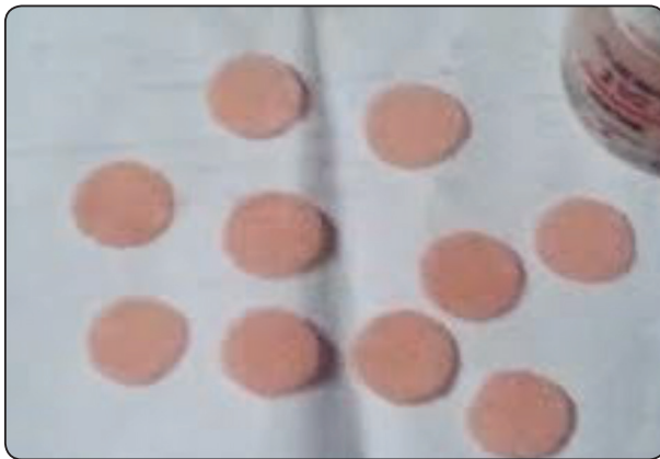
Fig. (1) disk specimen for color stability test.
