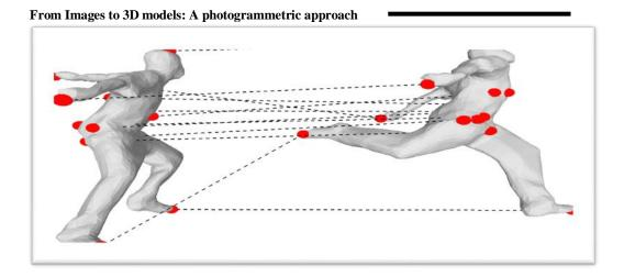
Figure 1. Illustration of point matching
