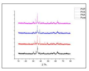
Fig. 2. XRD pattern to compare different polymers used in the preparation of copper ferrite
