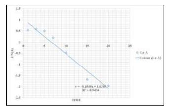
Fig. 4. First order reaction kinetics showing the calculating for rate constant.
