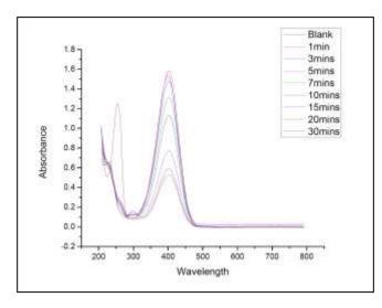
Fig. 3. UV-Vis chart sample to show the decrease in p-Nitrophenol peak at 400nm and the increase in p-Aminophenol peak at 300nm.
